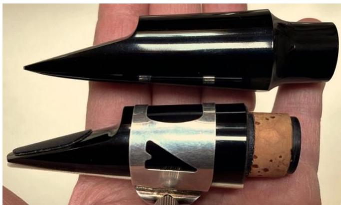
**PHOTO** shows the raw tenor MP and the clarinet modification after cutting the tenor on a lathe.
