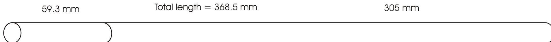
End correction of cylinder = .6 X 7mm = 4.2 mm      368.5 - 4.2 = 364.3 mm      364.3 - 305 = 59.3 mm
